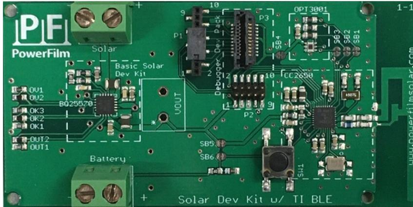
Figure 3, Assembled DEV-BLE-TI Circuit Board.
