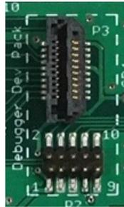
Figure 34, Circuit Board Dev Pack Connector.
