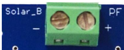
Figure 8, Solar input for charge control circuit 'B', DEV-BASIC.
