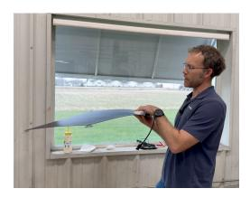
Don't over-bend. Cracking a cell won't kill performance entirely, but will reduce power output.
